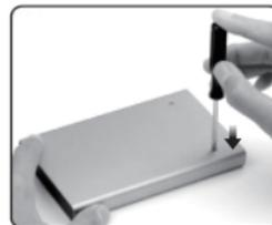
1. Detach the TPU frame, and unscrew the 2 screws at the bottom
