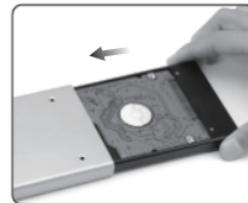
4. Slide back the middle frame and lock back the screws
