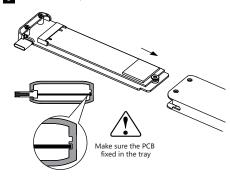
Push back the PCB tray in the aluminum case, and lock with screws
