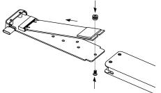
3 Install the M.2 SSD, and lock with screw
