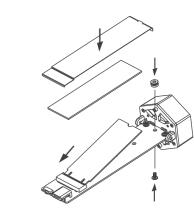
2 Insert the M.2 SSD, lock the screw to secure M.2 SSD, then attach thermal silicon pad.
